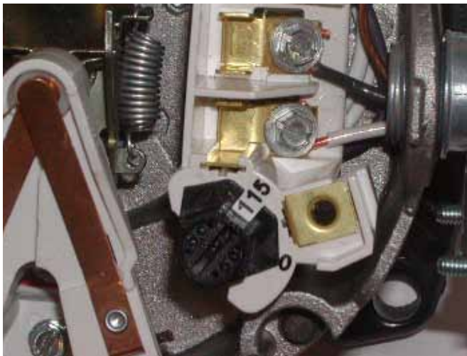
Figure 9 – Motor Set for 115 Volt Operation
